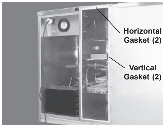
Figure 152. Gaskets on Rear of Filter/Fans Compartment
